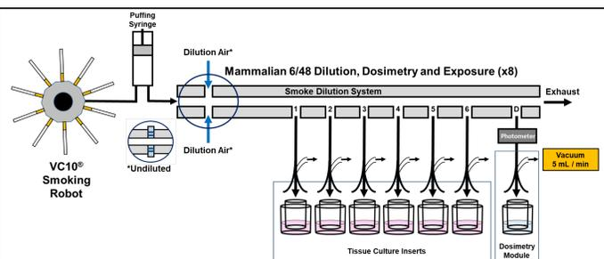
**Figure 1: Schematic representation of WA exposure system.** A Vitrocell® VC10® robot generated and delivered aerosols to the Mammalian 6/48 aerosol dilution and exposure system, with up to 7 concurrent doses plus a clean air control. The dosimetry modules allowed the capture and quantification of deposited aerosol constituents (nicotine, glycerol and carbonyls).
