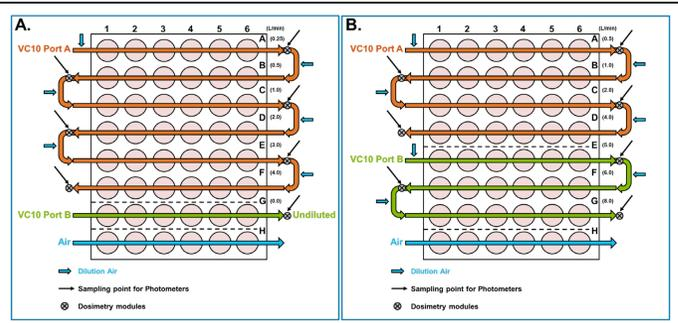
**Figure 2: WA exposure module.** Mammalian 6/48 WA exposure module set up for HTP (A) and combustible cigarette (B) exposures. HTP WA was serially diluted through rows 1 – 6 (0.25 to 4.0 L/min dilution airflows) or undiluted (0 L/min) in row 7. For combustible cigarettes, WA was serially diluted through rows 1 – 4 (0.5 to 4.0 L/min) and rows 5 – 7 (5.0 to 8.0 L/min). Row 8 (A & B) was used for air controls.
